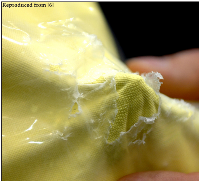
Resistance of STF-impregnated Kevlar under stab testing.
